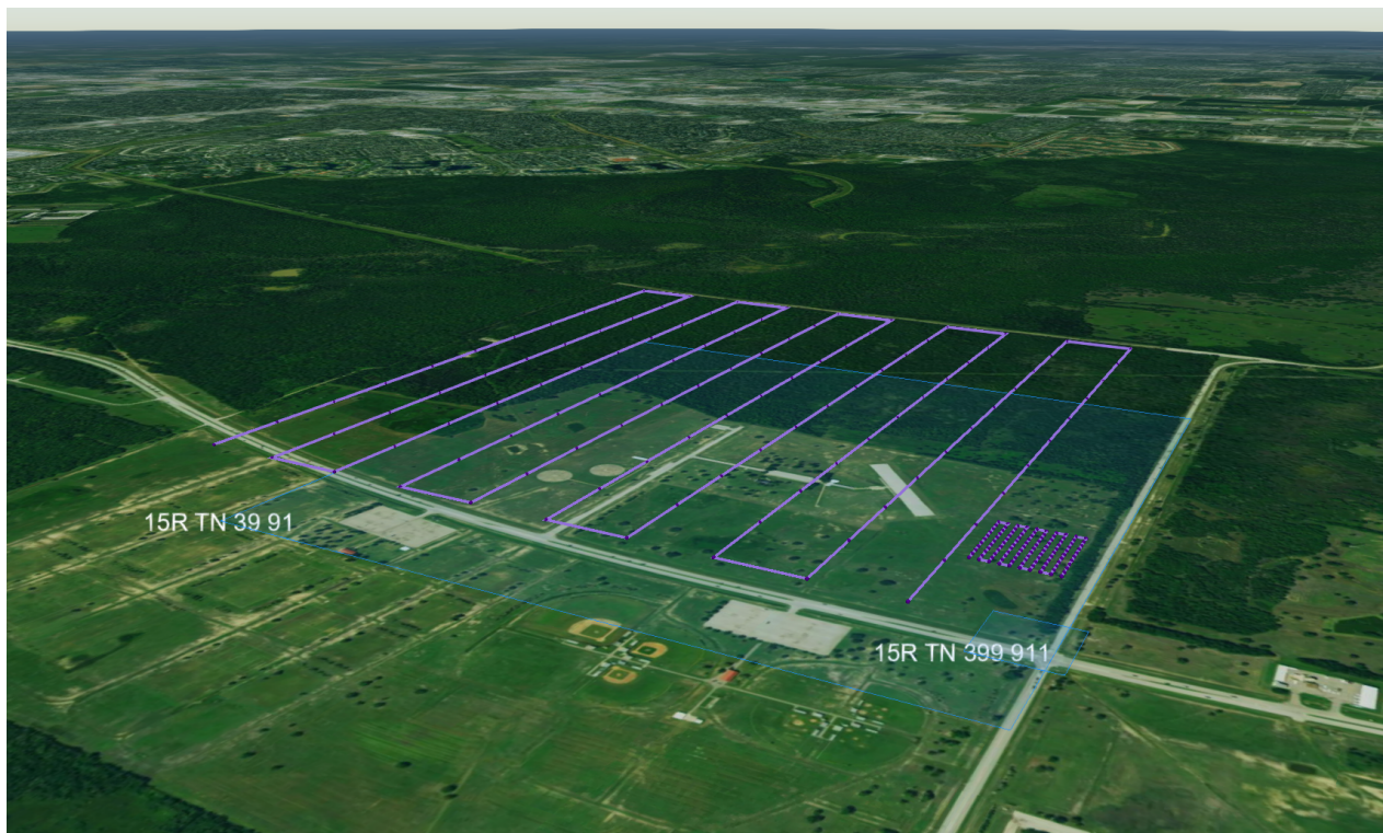
Waypoints and flight paths generated from USNG grids using UTM FLight Planner
